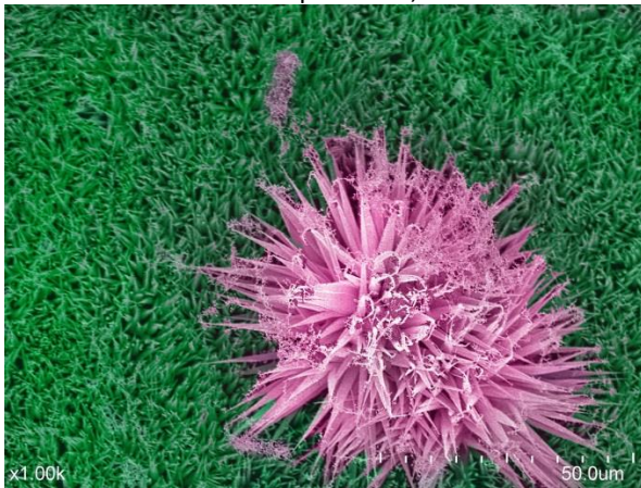
Crystallites in devitrified sodium borosilicate and annealed pyrolytic graphite glass composite
